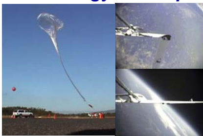
9/19/02: Unfolding & Transition Flight Test at 103,000 feet with 1/2-Scale Airplane (Mars relevant flight conditions)
