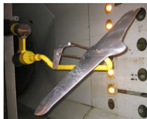
2004: Wind Tunnel Testing (1/4-Scale)
